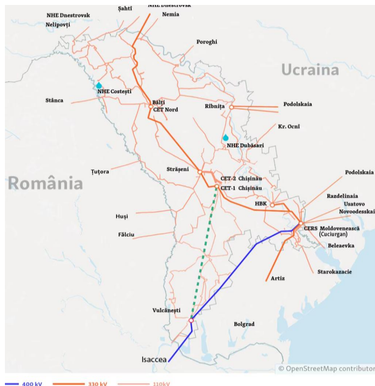
Fig. 11. The new 400 kV Vulcănești-Chișinău power line (in green) 97
